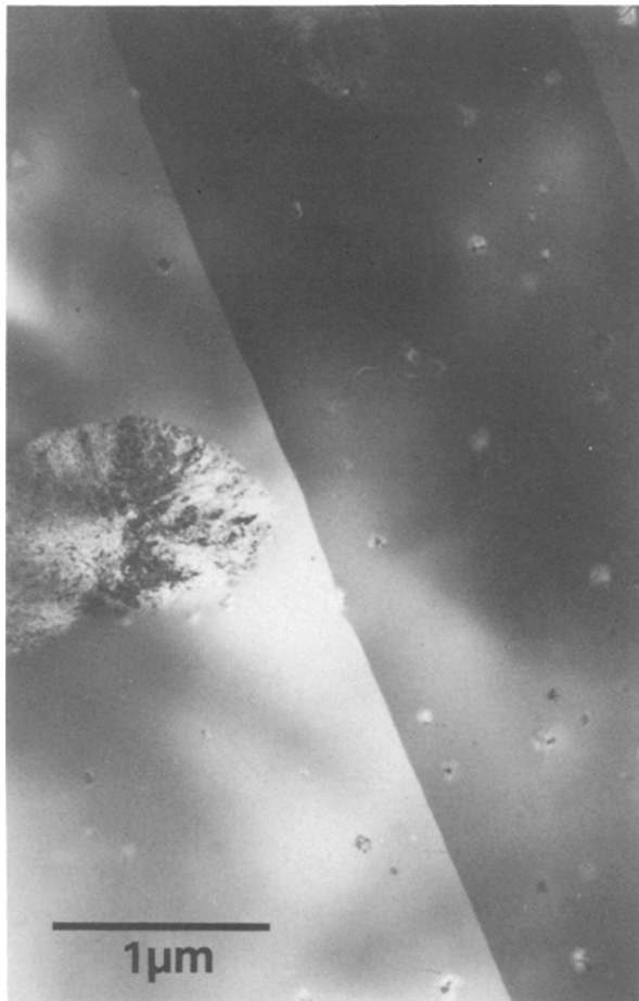
Figure 8 Shear bands in a slightly bent sample containing both eutectic and \tau -phase crystals. Thin foil for transmission microscopy was prepared from the tensile-stress side of the bent sample. Alloy C, after 6 min at 350°C.
